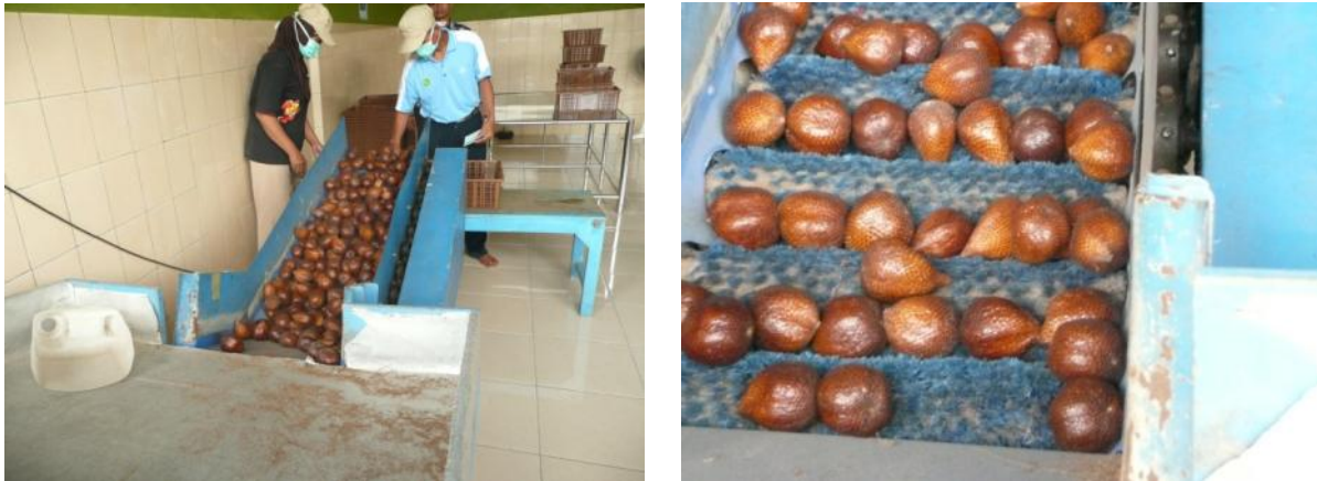
Figure 15 Fruit mechanically cleaned by passing over a conveyor belt fitted with brushes
